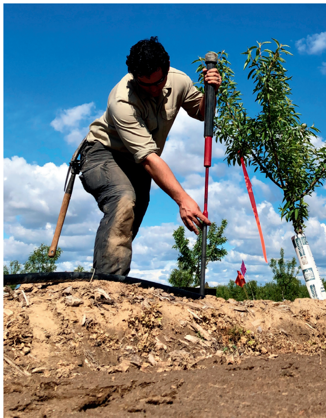
Slide hammer used to excavate bulk density cores. Photo credit: Cameron Zuber.
