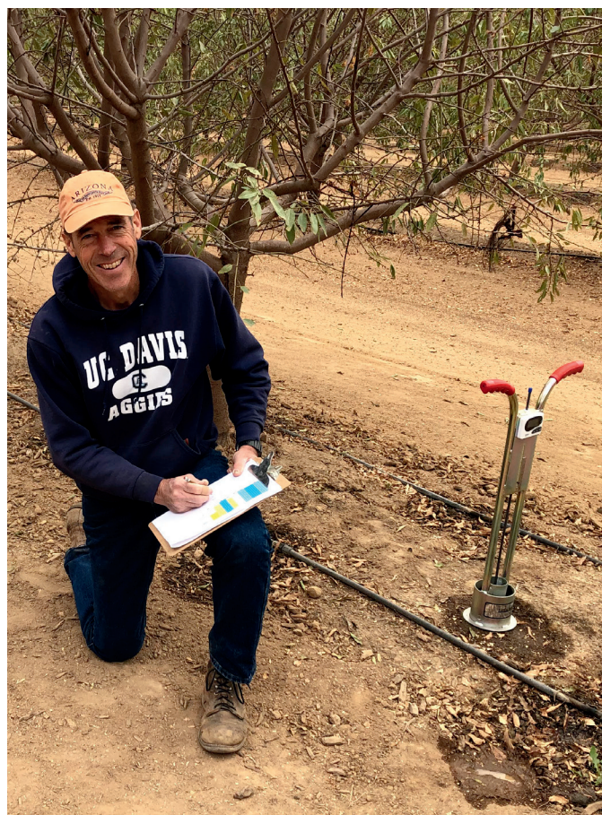
In-field soil infiltration measurement with a double ring infiltrometer.
