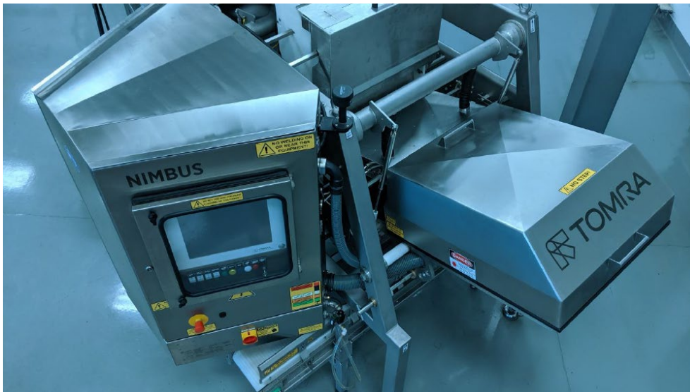
TOMRA Nimbus 640 with double Laser in DETOX ™ Configuration
